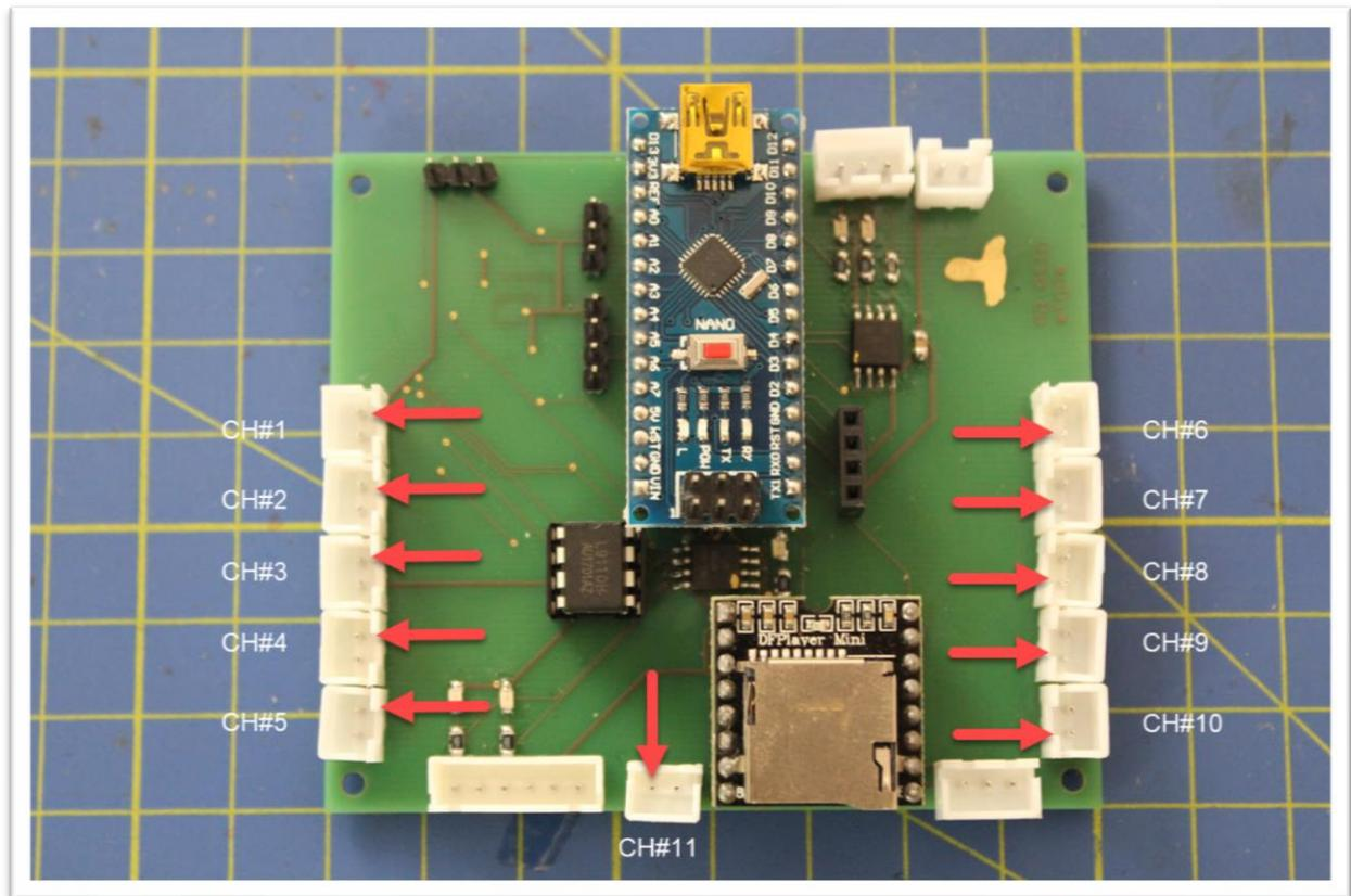
Figure 10 Kanal Anschlüsse
