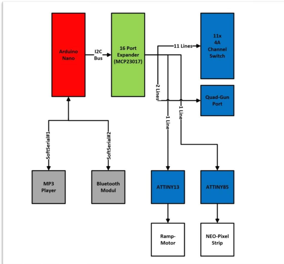
Figure 1 Board Diagramm
